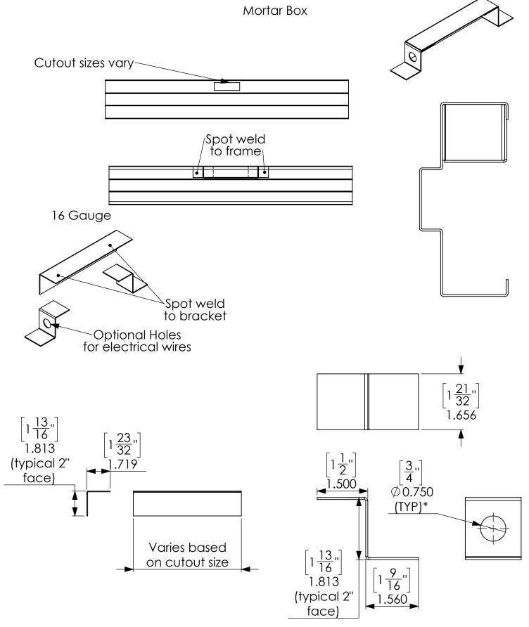
\*If conduit hole is needed, customer must specify if it is not 3/4" and conduit direction www.nationalcustomhollowmetal.com
